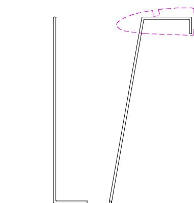
Landing gear from 0.6mm piano wire
